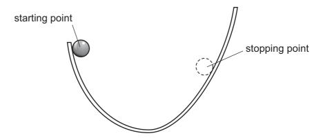
The ball is released. It rolls down one side of the track and part of the way up the other side. It then stops, before rolling back down again. The height of the stopping point is less than that of the starting point.
