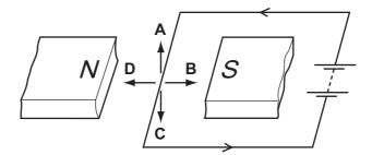
**34** A simple d.c. motor consists of a coil that rotates between the poles of a permanent magnet. The turning effect is increased by winding the coil on a metal cylinder.
