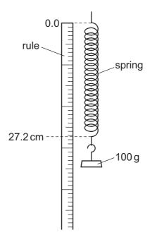
The 100 g mass is replaced with a 600 g mass. The length of the spring is now 89.7 cm. The spring has not reached the limit of proportionality.
