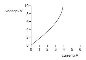
The voltage across the lamp increases. What happens to the temperature of the lamp and the resistance of the lamp?
